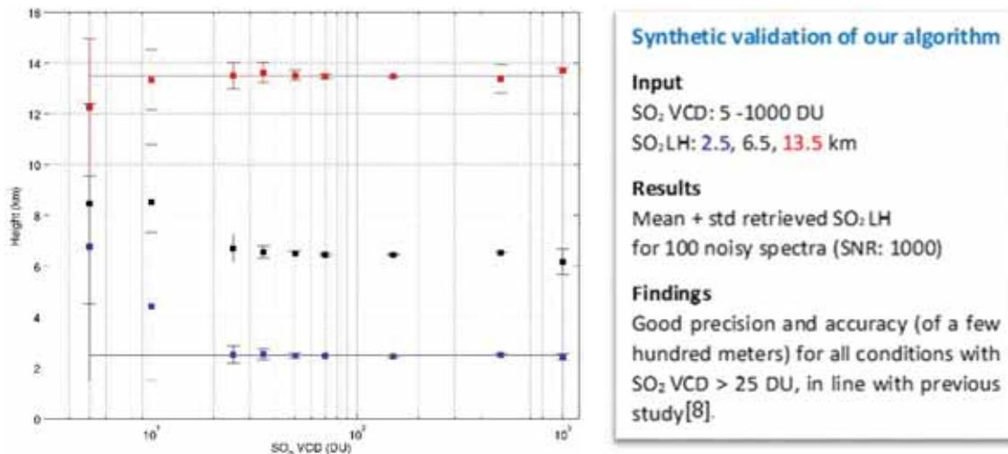
Figure 4: Illustration of synthetic validation of TROPOMI SO<sub>2</sub>LH retrievals (considering an O<sub>3</sub> VCD of 385 DU, a solar zenith angle of 30°, and an albedo of 5%).
