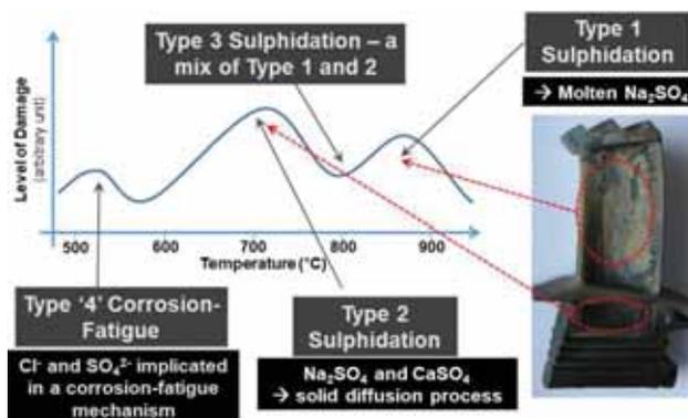
Figure 2: Illustration of the sulphidation mechanisms.
